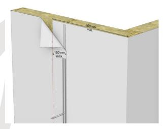
Figure 2 - External corner arrangement
