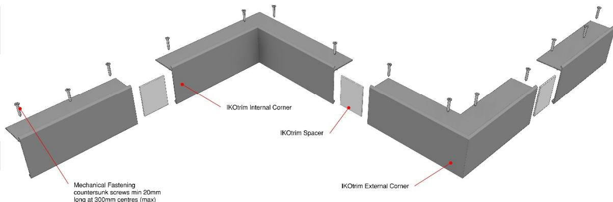
Any trim with a drip length of greater than 150mm must also be face fixed with mechanical fixings, to prevent wind uplift.
