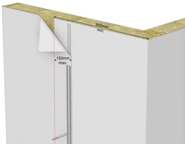
**Figure 2 - External corner arrangement**
