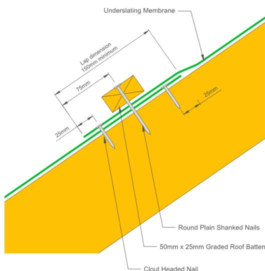
**Figure 2: Creating the Overlap - Battened Overlap Detail**
