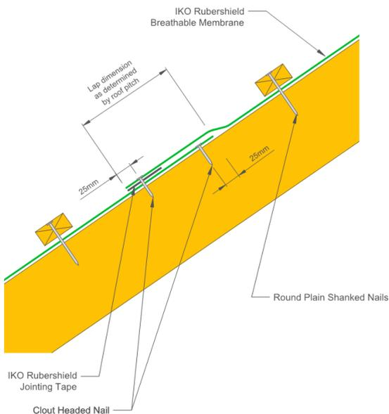
**Figure 1: Creating the Overlap – Taped Detail**
