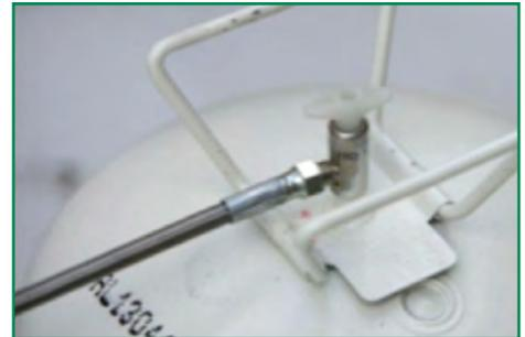
Image 1: Canister with the braided-hose correctly attached
