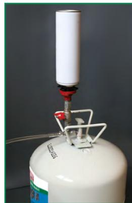
Image 7: Screw Cleaning Aerosol into the adaptor
