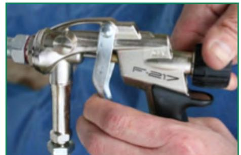
Image 3: Black valve to adjust bead width
