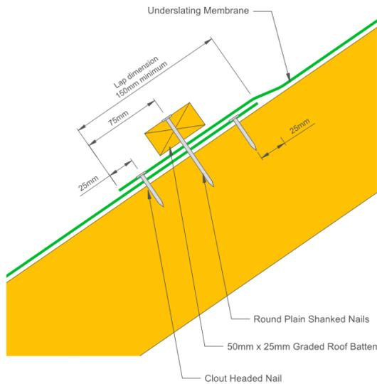
**Figure 1: Creating the Overlap - Battened Overlap Detail**
