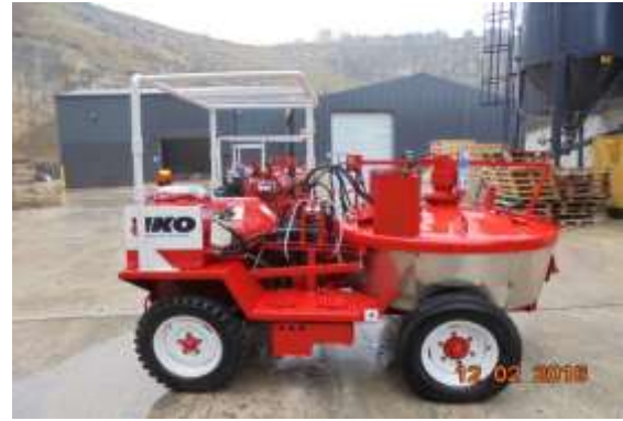
Luggers for transportation to point of lay
