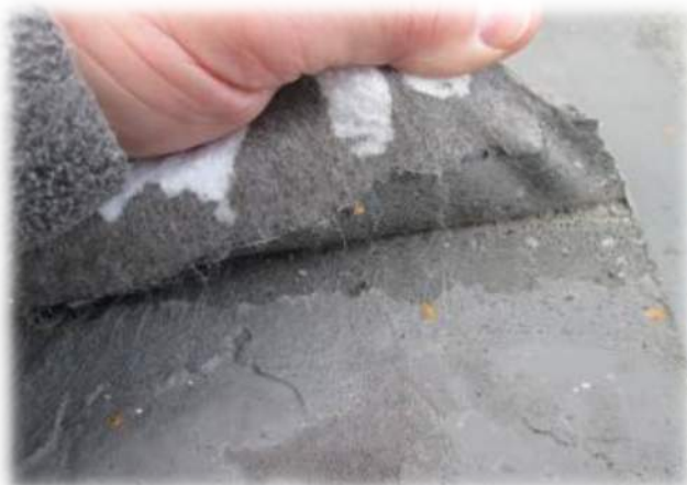
A good adhesion will require some amount of force to remove the test sample.
