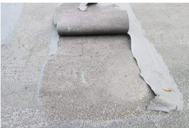
Pull free end. Should the coating be freely removed from the substrate then a primer should be considered and re tested.
