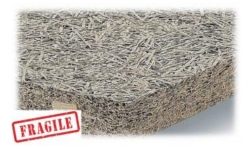
It was used generally during the 1960s until the late 1990s to provide insulation as well as a structural roof decking; it was also used as a permanent shutter to insitu concrete.
