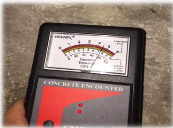
Moisture content reading should be within 6%
