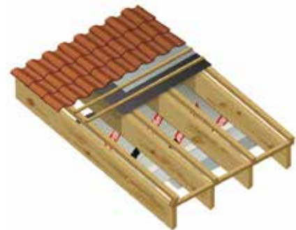
Under rafters ventilated
