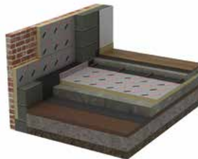
Above ground bearing slabs
