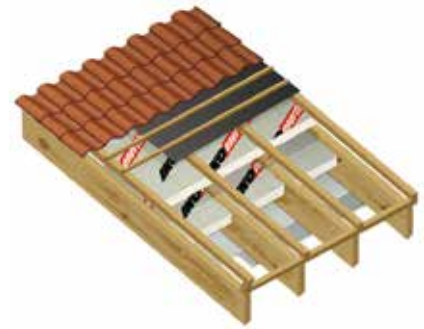
Over and between rafters
