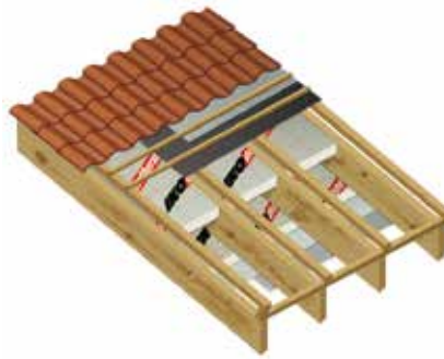
Between and under rafters ventilated
