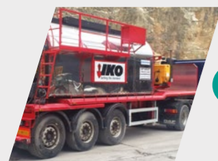
Permascreed delivered to site in purpose-built hot charge vehicles
