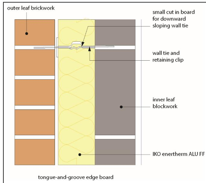
A.7 The corresponding edges of the two interlocking boards are cut with a sharp knife or fine-toothed saw to allow insertion of the wall ties so that they are sloping downwards to the outer leaf. Care must be taken to ensure that damage is minimised during this process.
