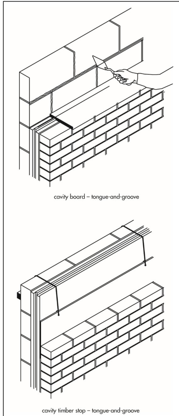
A.13 The boards can be cut using a sharp knife or fine-toothed saw to fit openings, eg around windows, doors and airbricks. It is essential that cut pieces completely fill the spaces for which they are intended and are adequately secured.
