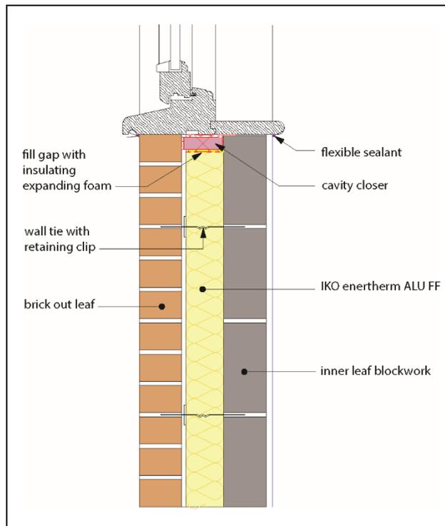
A.16 Additional wall ties at 300 mm vertical centres within 225 mm of all openings are recommended in BS EN 1996-1-1 : 2005 and BS EN 1996-1-2 : 2005. For the product, this would involve piercing the boards and may introduce an unacceptable risk of water penetration. Therefore, an additional wall tie should be included within 225 mm of the opening on each board course level to satisfy the structural requirements of the wall (see Figure 6).
