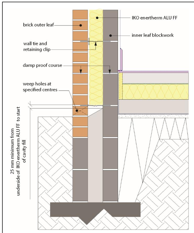
A.5 The internal leaf is then built up to a course above the next row of wall ties, which are placed at spacings of 450 mm vertically and (not more than) 900 mm horizontally (see BS EN 1996-1-2 : 2005). Excess mortar must be cleaned from the cavity face of the internal leaf.
