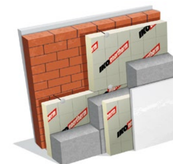
Partial fill with insulated plasterboard
