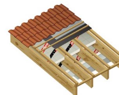
Between and under rafters ventilated
