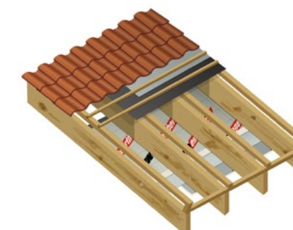
Under rafters ventilated
