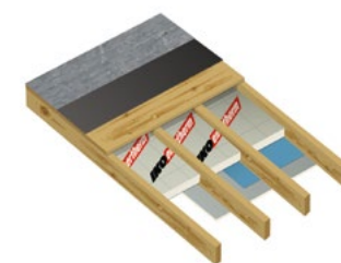
Cold roof IKO build-up
