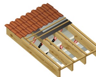
Between and under rafters unventilated
