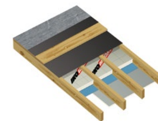
Cold roof typical build-up
