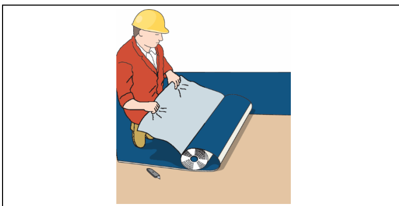
Figure 1 Membrane laying process
