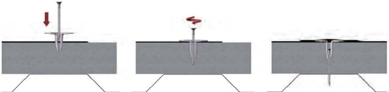
1. Lightly insert the washer and IKOfix Stainless Steel fastener into the insulation board.
