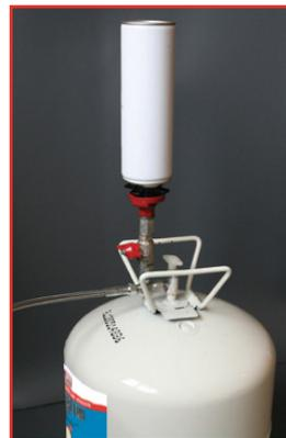
Image 10: Screw Cleaning Aerosol into the adaptor
