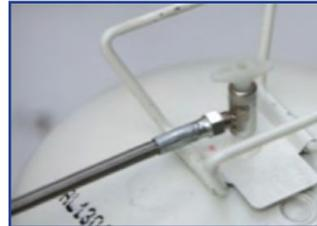
Image 1: Canister with the braided-hose correctly attached
