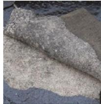
**Failed peel test - easily pulled from the substrate**
