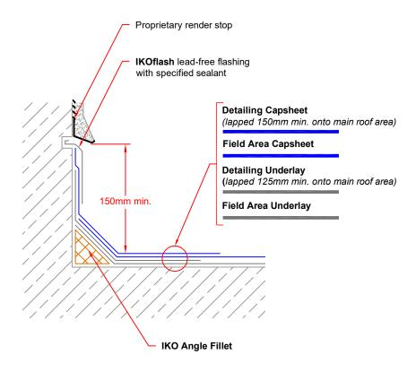
**Note:** Detail to illustrate lapping & waterproofing arrangements in relation to IKO specified roofing system. The client / Contractor is to confirm with relevant parties any limitations or restrictions of vertical application in relation to Building Regulations Approved Document B prior to works.
