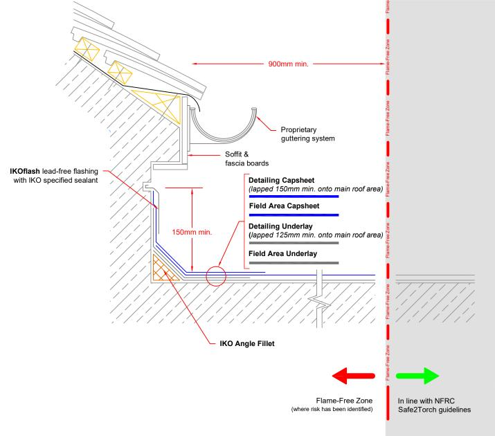
Additional mechanical fixing through the membrane at the top edge to resist slippage will be required on vertical details >250mm.
