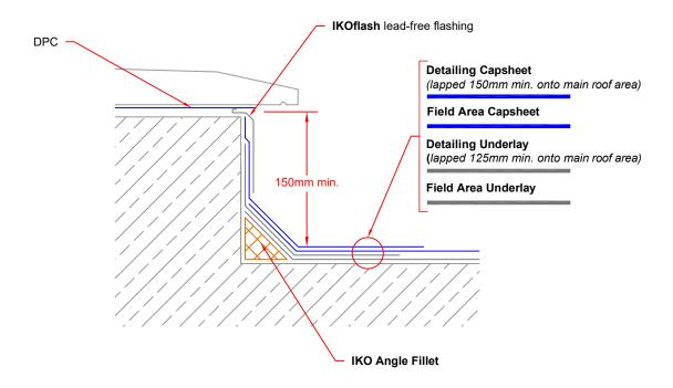
**Note:** Detail to illustrate lapping & waterproofing arrangements in relation to IKO specified roofing system. The client / Contractor is to confirm with relevant parties any limitations or restrictions of vertical application in relation to Building Regulations Approved Document B prior to works.
