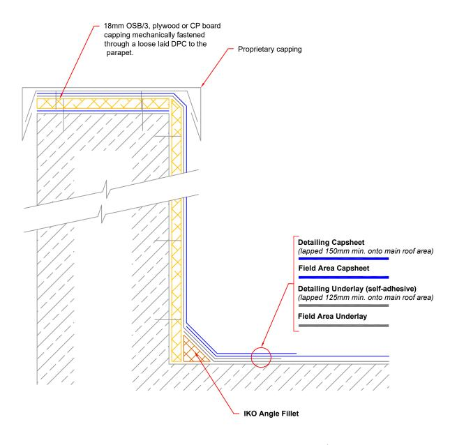
Note: Detail to illustrate lapping & waterproofing arrangements in relation to IKO specified roofing system. The client / Contractor is to confirm with relevant parties any limitations or restrictions of vertical application in relation to Building Regulations Approved Document B prior to works.
