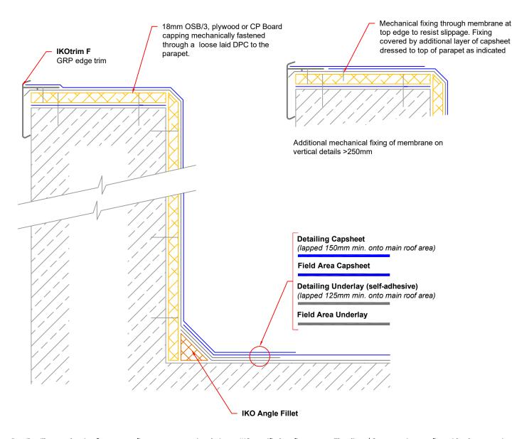
**Note:** Detail to illustrate lapping & waterproofing arrangements in relation to IKO specified roofing system. The client / Contractor is to confirm with relevant parties any limitations or restrictions of vertical application in relation to Building Regulations Approved Document B prior to works.
