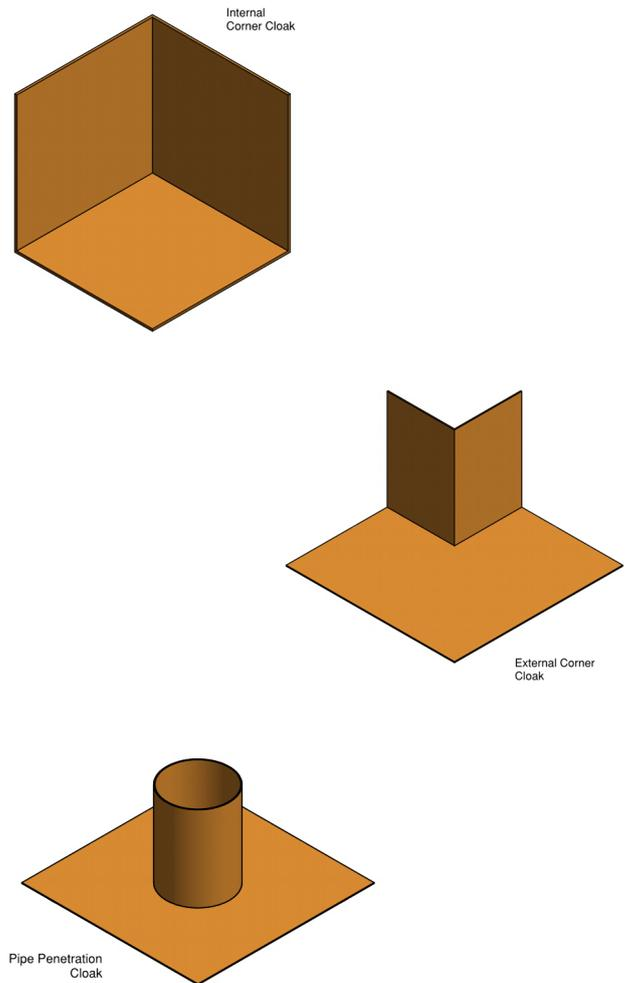
Figure 1 – IKO Hyload Pre-formed Cloak Units
