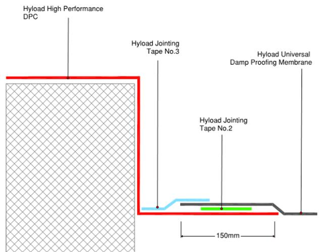
Figure 4 – Formation of Sealed Overlap with Perimeter DPC
