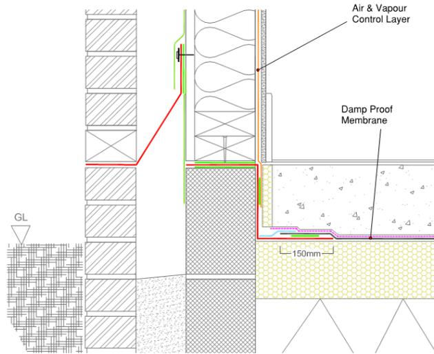
Figure 2 – Damp Proofing Applications
